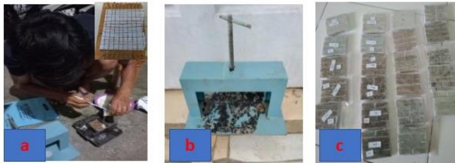
Figure 3. Composite manufacturing process. (a). Pouring of the resin mixture and CaCO 3 , (b) Composite pressing, and (c) Composite samples ready for testing.
