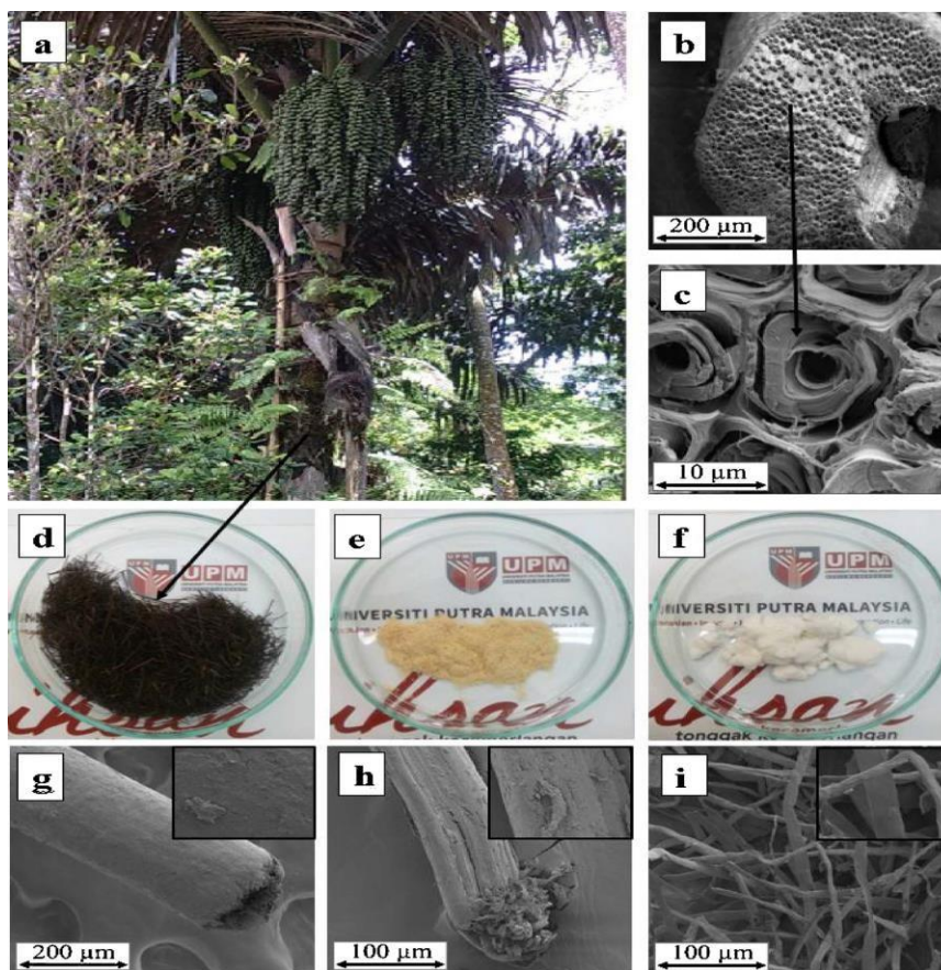
Figure 1. Photographs of (a) the sugar palm tree, (d) raw sugar palm fibers, (e) bleached fibers and (f) alkali-treated fibers; FESEM micrographs of sugar plant fibers: (g) cross-section, (b)longitudinal section, (c) primary, secondary cell wall and middle lamella, (h) alkali-treated fibers, (i) and bleached fibers [12]
