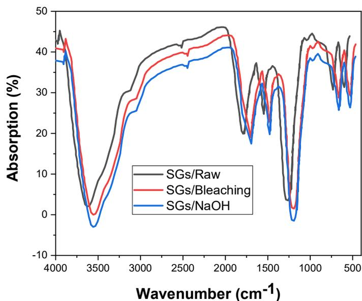
Figure 4. FTIR of *S. grandiflora* fibers (SGs) with different treatments.
