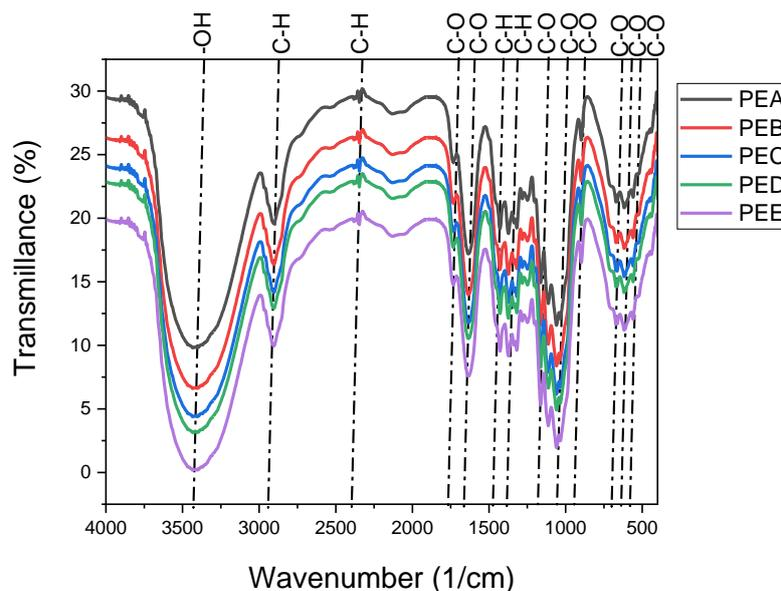
Figure 5. FTIR of WPH/RH reinforced composite polyester
