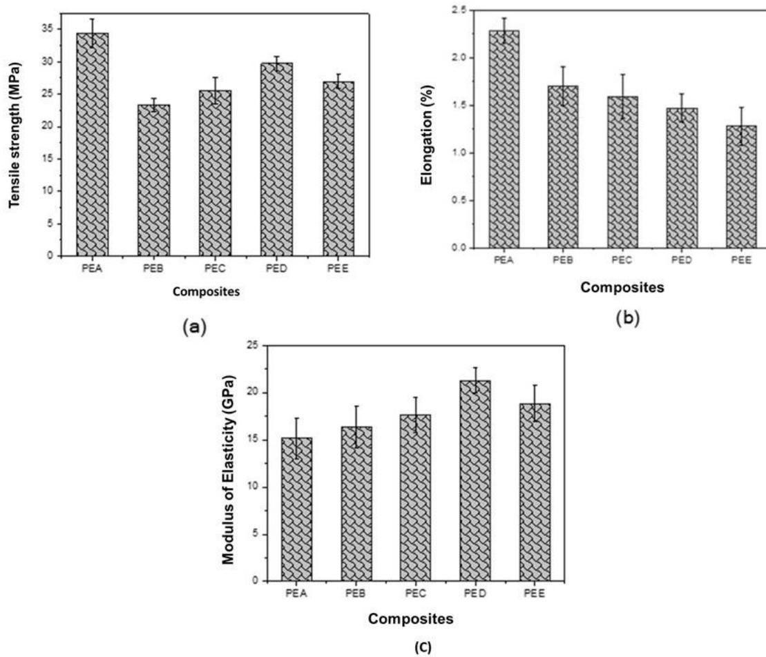
Figure 6. (a) Tensile strength, (b) Elongation, and (c) Modulus of elasticity of water hyacinth powder/rice husk reinforced composite polyester
