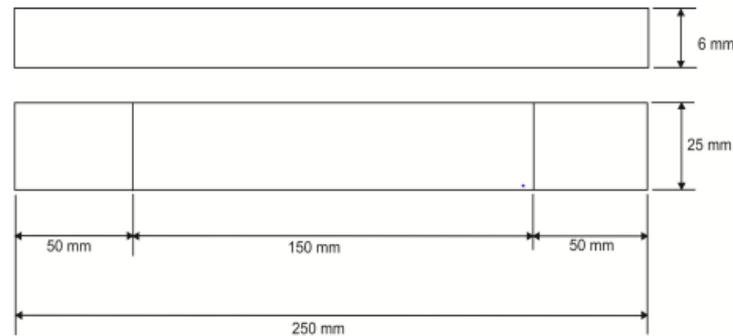
Figure 4. Schematic of ASTM D3039 tensile strength test samples.
