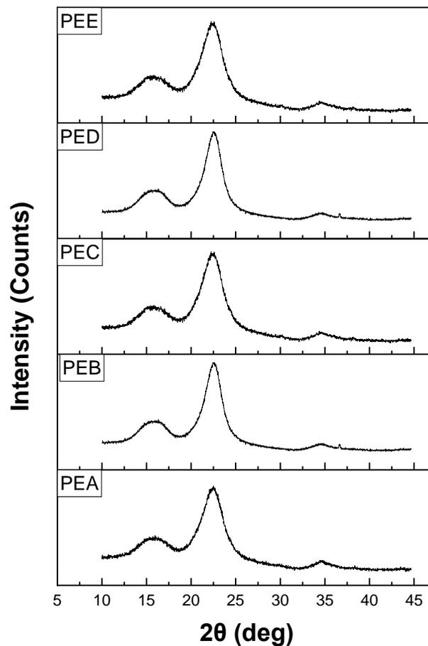
Figure 7. XRD of WPH/RH reinforced composite polyester
