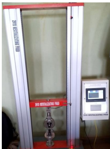
Fig 4. Universal material Testing Machine (100 KN capacity)
