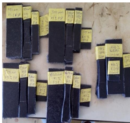
Fig 3. Cut samples to undergo Physico-mechanical Testing
