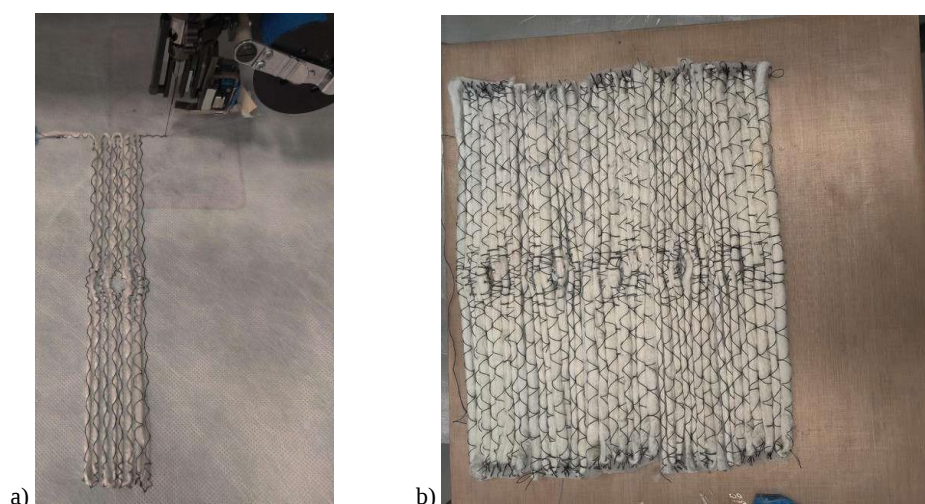
Fig. 6. a) showing FULL TFP pattern as made in the Laystitch machine b) showing FULL TFP samples placed in mold.
