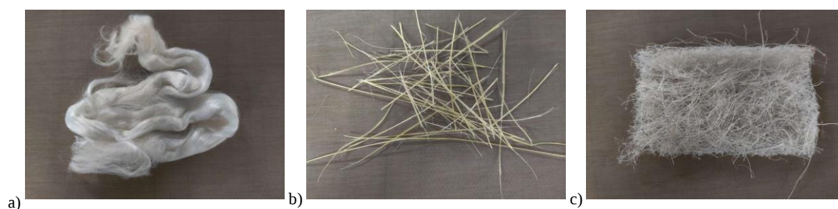
Fig. 1. Different types of bamboo fiber used in study, with a) being the VBF, b) being showing the MBF and c) showing the CBF
